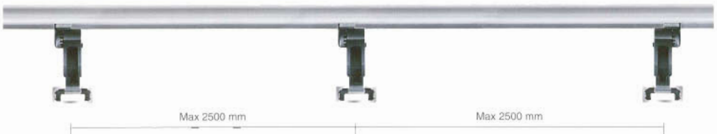
Below: The distance between the C-shaped profiles must not exceed 2500 mm.
